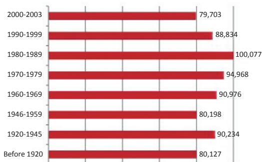
Average Annual Energy Consumption in BTUs (British Thermal Units), commercial buildings. (US Energy Info. Agency, 2003)
