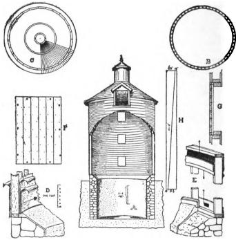
Fig. 328—construction of silo in detail
