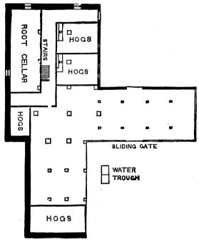
Fig. 18—PLAN OF BASEMENT
