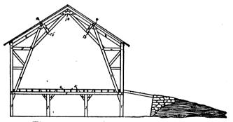
Fig. 3—INTERIOR BENT OF A BASEMENT BARN
