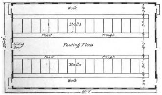
Fig. 84-FLOOR PLAN OF A SANITARY COW BARN
