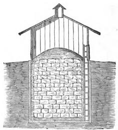
Fig. 248—section of underground ice house
