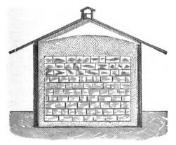
Fig. 240—section of an ice house filled
