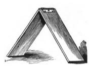
Fig. 236—SECTION OF CRIB Fig. 237—BOARD RAFTER
