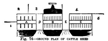
are poles eight feet long. They rest at the foot on the cross piece at the middle of the post, and are halved in and spiked to the post, and the upper end supports the plate in the middle. Figure 74 shows the ground plan, on which 1, 2, 3, 4,  $\tilde{s}$  and  $\tilde{s}$  are lots opening into all the fields on the farm; 7 is the cistern, A is for sheep, B and
