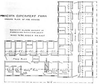
Fig. 151-GROUND PLAN OF MINNESOTA HOG BARN
