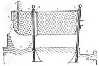
Fig. 79—cross-section of improved cow stall
