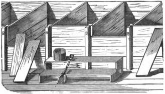
Fig. 290—ARRANGEMENT OF BINS IN GRANARY
