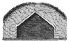
Fig. 337—cross-section of a root cellar
