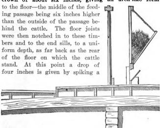
Fig. 63-SECTION OF STALL WITH FEEDING APPARATUS
