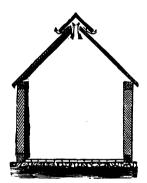
Fig. 246—VERTICAL SECTION OF ICE HOUSE
