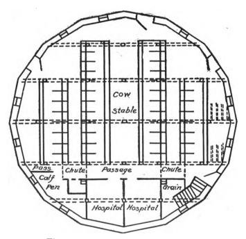
Fig. 9—arrangement of the basement
