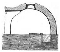
Fig. 282—SECTIONAL VIEW OF SPRING HOUSE
