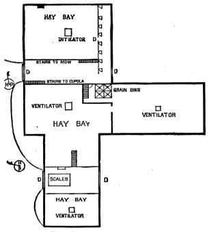
Fig. 16—PLAN OF HAY FLOOR
