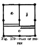
one foot in the ground, and project as far above the surface. They are arranged as in Figure 179. Four by fourinch sills are laid upon the posts, with a cross sill in the center, and halved together at the joints. No wall posts are used, the stout boarding being made to serve the purpose. The structure is eight feet each way, or can be made when
