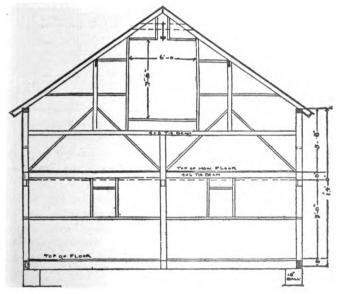
Fig. 39—END ELEVATION OF FRAMING
