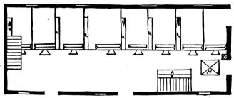
Fig. 164—PLAN OF MAIN FLOOR OF PIGPEN
