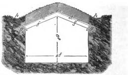
Fig. 346—cross-section of a field root cellar
