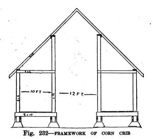
corner to plate so as to resist wind pressure or weight of grain settling unevenly. Siding need not be matched stuff unless snow blows into cracks of buildings. In many sections it is customary to board up with six-inch stuff and leave the cracks slightly open. This crib is as strong and durable as it need be for any region. The length will depend on the conditions involved. The crib is all of two-inch stuff nailed and spiked together.
