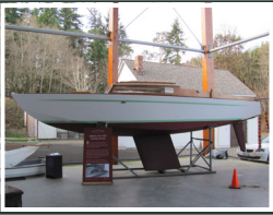
THUNDERBIRD 1 The hull of Thunderbird 1, a plywood sloop designed by naval architect Ben Seaborn and built by Ed Hoppen, is on display at the Harbor History Museum in Gig Harbor. The sloop features a v-shaped hull allowing for the stiffness of multilayered plywood.
