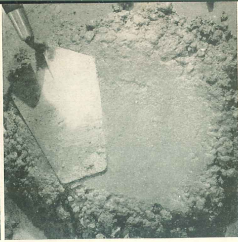
Center —A good concrete mix for most farm jobs looks like this. Note that the mix is fairly stiff, yet, because of proper proportioning there is a generous amount of cement-sand mortar to make smooth, dense concrete surfaces. There are few farm jobs that should have a wetter mix than this.
