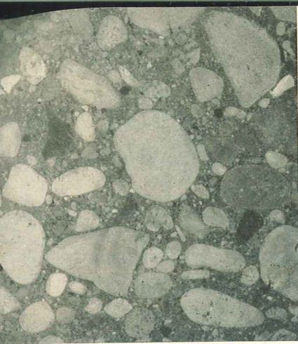
Left —Most economical and most durable concrete is obtained only if proper amount of gravel is used in the mix. Gravel used however must be properly graded. See photograph and explanation on pages 5 and 6.
