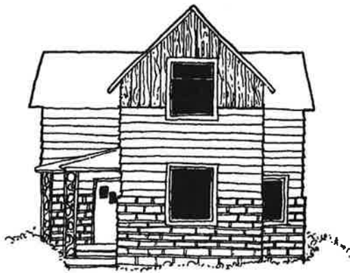
Replacing historic lapped siding with wood shingles is non-compatible.
