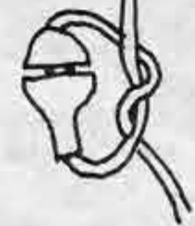
Tie a knot like this connecting drill cord to extension cord so it won't slip out when you pull on it.
