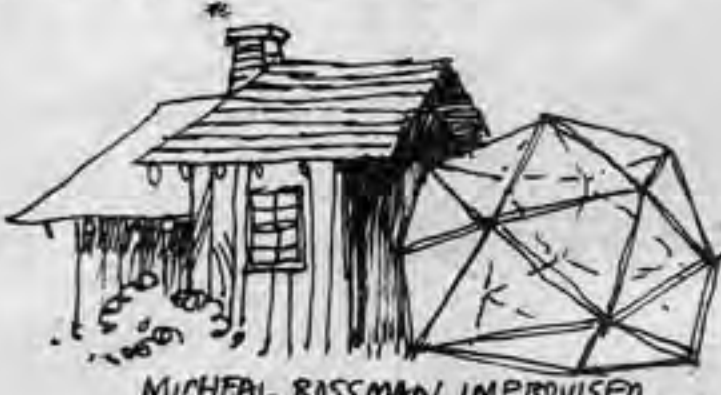
MICHAEL ROSSMAN IMPROVISED A 1X2 AND POLYETHYLENE CRYSTAL ROOM ON THE SIDE OF HIS WOOD HOUSE IN BERKELEY
