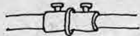
The curved sections of pipe were joined together using standard screw unions.
