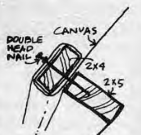
CANVAS ROLLED UP OVER OPENINGS TO ACT AS GUTTER
