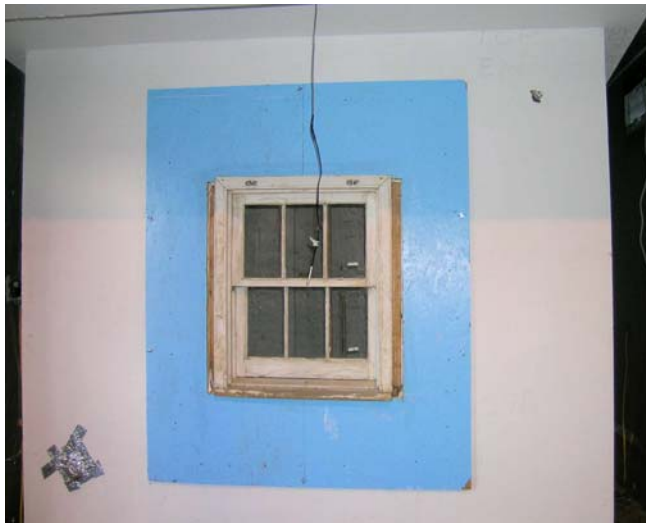
Figure 2-11. Test cell configured to test small double hung window
