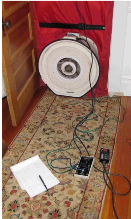
Figure 2-7. Blower Door Installed in Bedroom (Speed control on floor on right; digital manometer in center)
