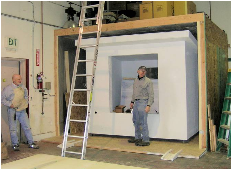
The photo on the left shows three walls of the chamber completed with the test cell inside. The outer chamber, likewise well insulated and sealed, is cooled while the test cell is heated to test U values.
