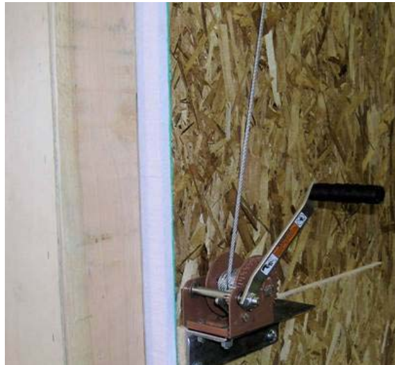
The technical team constructed a 380 pound door (see photo at left), insulated with both fiberglass and polyisocyanurate to R-25. The photos below show a winch and pulley system, suspended from steel roof rafters, used to open and close the chamber door.
