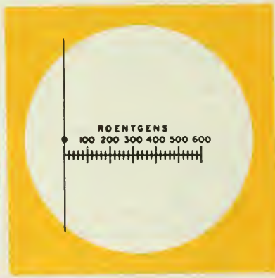
Enlarged view of a dosimeter scale. The instrument is used to measure the total amount of radiation to which a person has been exposed.
