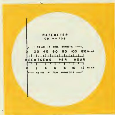
Enlarged view of a ratemeter scale. This particular model must be exposed to radiation for certain specific times to measure the dose rate (intensity) of radiation.
