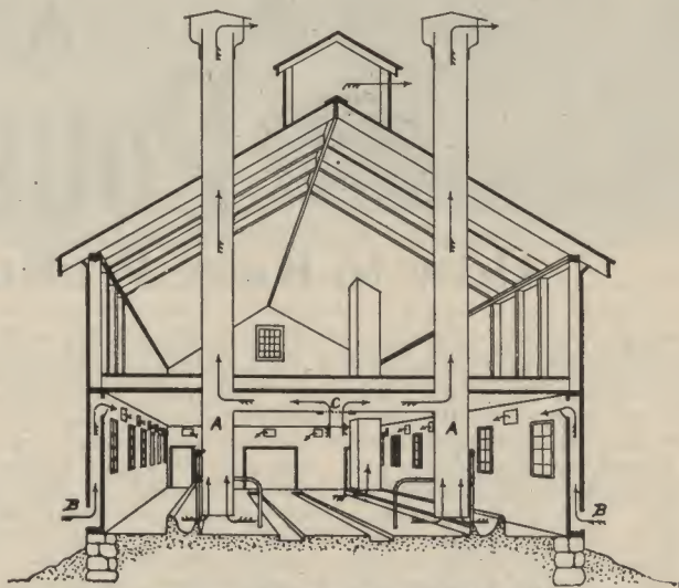
FIG. 1. VENTILATING SYSTEM FOR BARN
