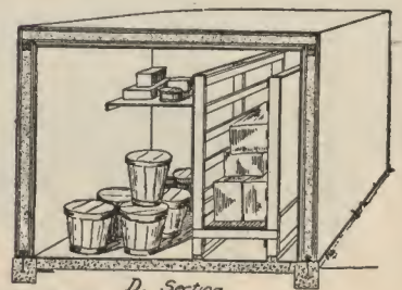
Diagrams showing cross section and details of construction of a farm refrigerator: A, Detail of wall construction and ice bunker; B, front elevation; C, floor plan; D, sectional view.
