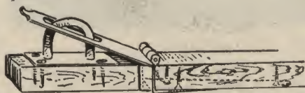
Back Leaf is Bent and Screwed from Inside.
