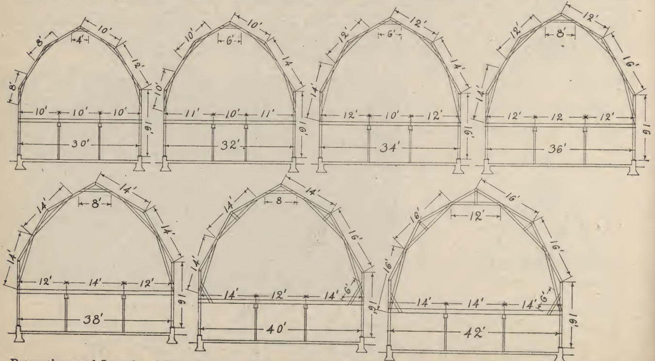
Proportions and Lengths of Barn Framing Members for Strong, Neat Gambrel Roofs for Barns of 30 to 42-Ft. Spans
