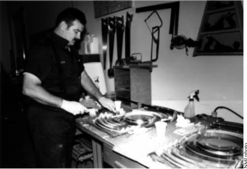
**Figures 37 and 38.** Joe Cocking (above) and Nick Johnston (below) restore a classical lens at the U.S. Coast Guard Exhibit Center.
