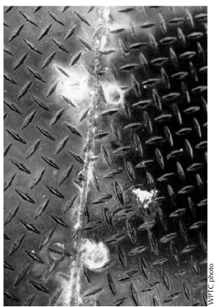
**Figure 7.** The white chalky residue around the steel bolt heads on this aluminum deck is the by-product of the corrosion occurring at these connections.
