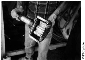
**Figure 33.** Close-up of the studded flaps mounted on the rotating head. To use the tool, it is held against the face of the iron member and as the studded flaps spin they "slap" the surface and "knock" the paint off the iron.
