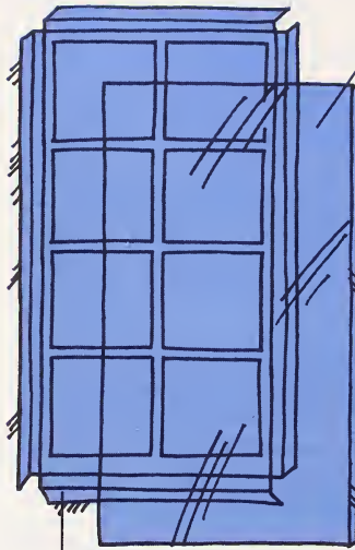
The plastic frame snaps open and shut for easy insertion of plastic.
