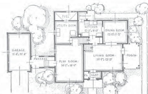
FIRST FLOOR AND BASEMENT PLAN
