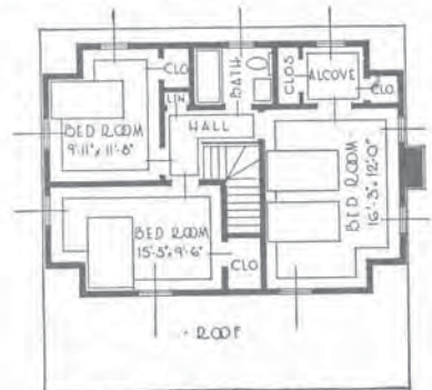
SECOND FLOOR PLAN If second bathroom is needed, it will work out nicely in alcove and closet space.
