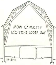
CROSS SECTION—A GAMBREL ROOF SHAWVER TRUSS
