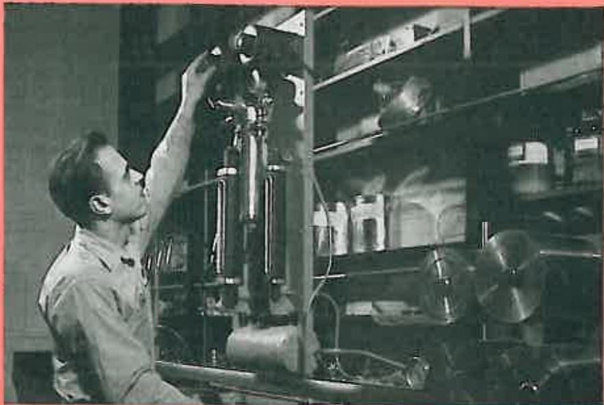
One section of the new Research Center is devoted to the development of better brushes. Here, an assistant adjusts a fixture on the fiber drawing machine used in making synthetic brushes. PPG research was responsible for development of synthetic Neoceta bristle.
