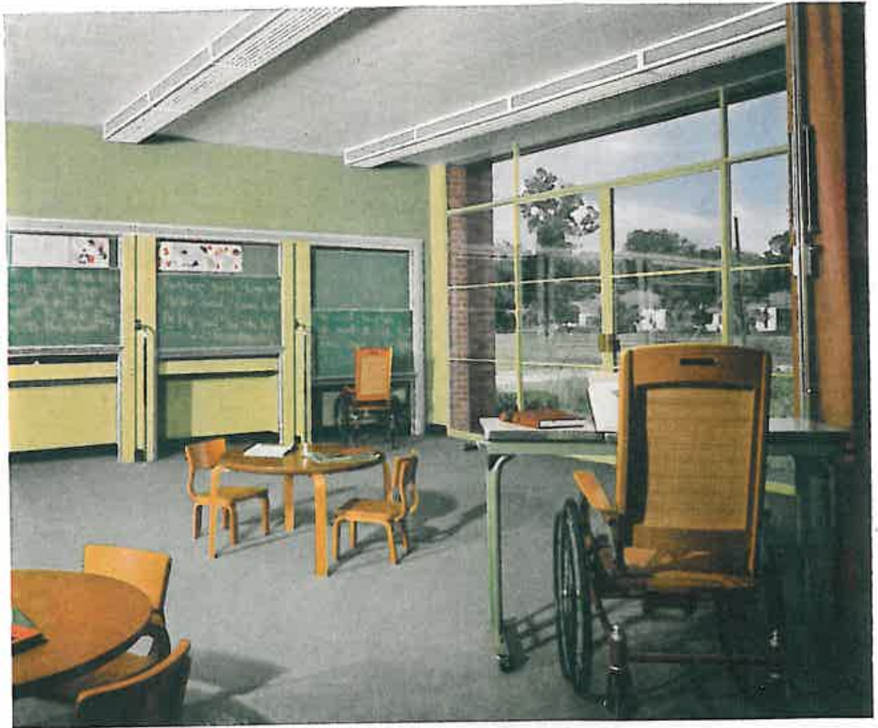
Colorful classroom features an "open" PPG glass wall treatment and chalkboards which may be adjusted to wheelchair height.
