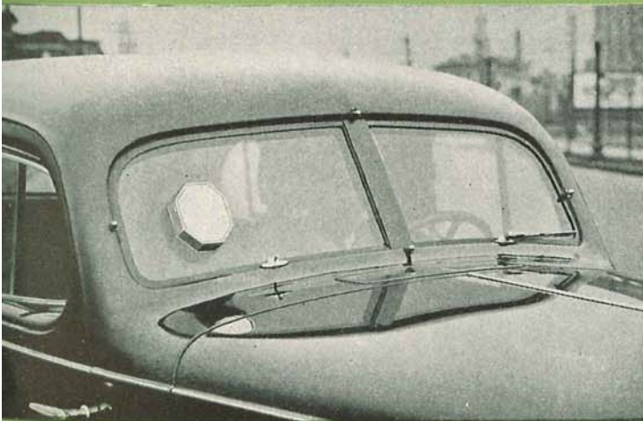
A typical Multiplate-equipped Police Cruiser showing Multiplate windshield and windows pierced with gunports.
