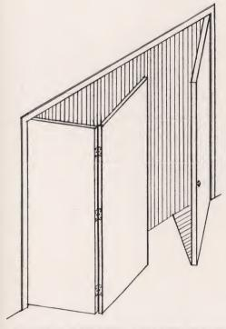
DOUBLE OPENING GARAGE DOOR Made by Hinging Three Flush Exterior Doors Vertically
