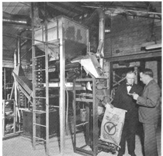
Fig. 1.36—The crushed glass, or flake, passes through magnetic separators, and then is discharged into bags.
