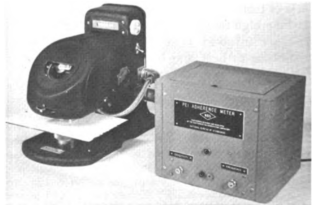
Fig. 1.44—PEI adherence meter. The electronic components are contained in the box at the right. A white 4" x 6" enameled metal specimen is in position for adherence evaluation following the deformation treatment. The deformed area of the specimen has been covered by lowering onto it the meter head containing over 150 probes, individually spring mounted. The test determines the percentage of the deformed area that retains sufficient enamel to prevent contact of the probes with the basis metal. At a "go" signal, the adherence meter automatically scans the probes and records the number of them that are in electrical contact with the metal. The results are converted into terms of "adherence index" by a simple mathematical formula.
