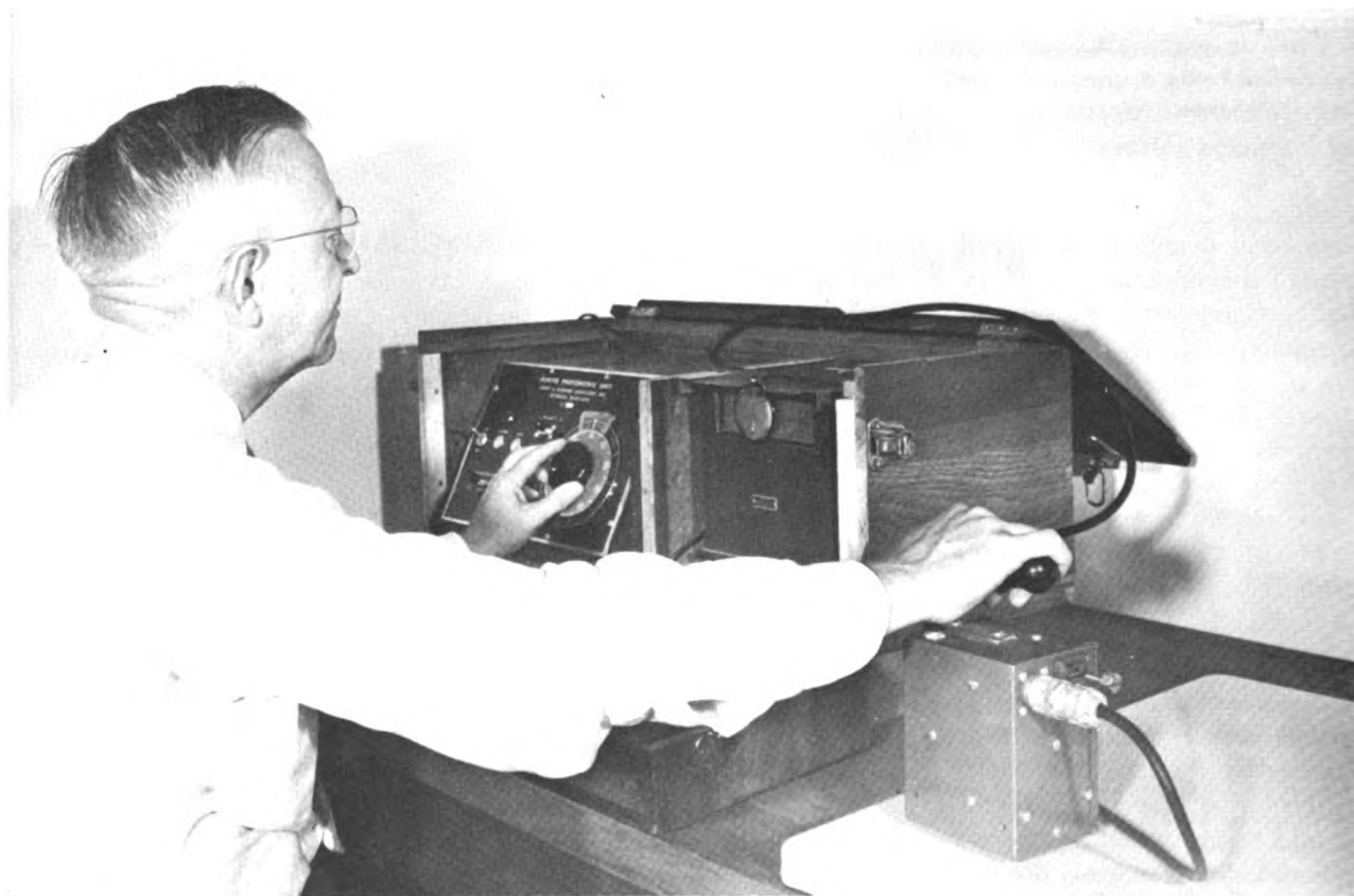
Fig. 1.46—One type of glossmeter. The white porcelain enameled steel panel being tested for specular gloss is at the lower right, and the gloss-head of the apparatus (which contains a light source) is being held in place by the operator. The fraction of incident light that is reflected, as by a mirror, is measured with the aid of photoelectric cells.
