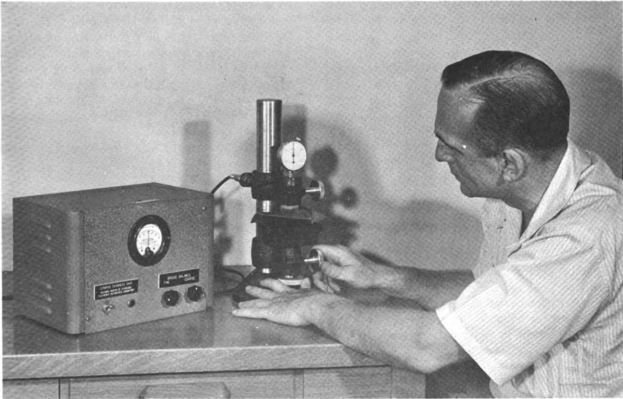
Fig. 1.45—Coating-thickness gage. Used for measuring thickness of ceramic coating on non-magnetic metal. The instrument is described in reference 9. The specimen being tested is a turbine blade with a fir-tree type of root, that is visible at the right, below the upper knob. When the test head is in contact with the surface of the coating the instrument indicates the coating thickness, by virtue of variation in the inductance of a coil in the head with its distance from the metal in the specimen.
