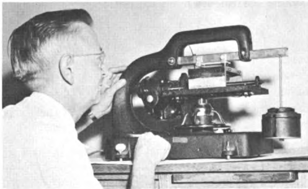
Fig. 1.50—Gouge-resistance test equipment. The load on the end of the lever is transmitted to the face of an enameled metal specimen (not visible) through a 3/32 " steel ball under a hardened steel plate attached to the lower side of the lever. The specimen-support is moved slowly by a motor-driven worm gear, causing the loaded ball to roll on the specimen. The load required for the ball to gouge the enamel determines the "gouge resistance" of the specimen.
