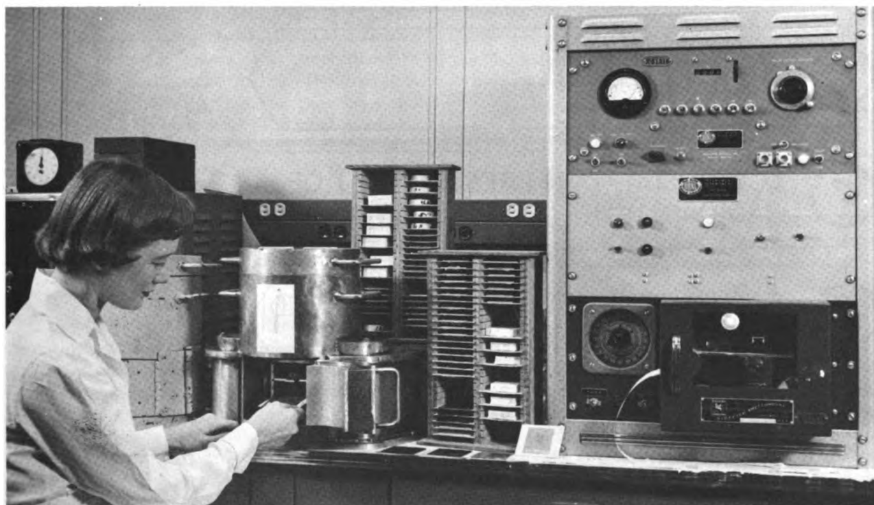
Fig. 1.26—Use of a G-M Counter For Measuring Radioactivity on Contaminated Porcelain Plates.
