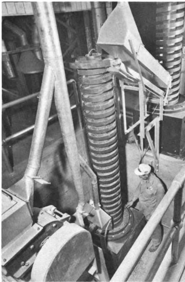
Fig. 1.35—The glass passes along on a conveyor, through a crusher (lower left corner), and then over two Syntron vibrating cooling conveyors.
