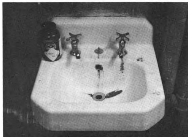
Fig. 1.25—Example of Failure of a Non-Acid Resisting Porcelain Under Improper Use.
