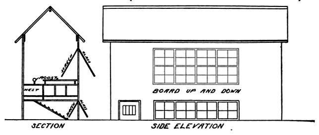
This little house is four feet wide and twelve feet long with a scratching shed the full size on the ground under the floor. This space underneath is two feet high and the windows should extend well across the front side.
