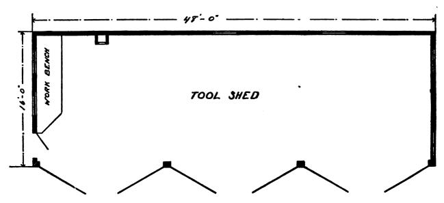
but you don't need so much height to the back end. The doors in this plan are ten feet high and the cross girts are the same height because it is sometimes necessary to move the machines lengthwise of the shed and the same head room is then needed. A truss is formed at each bent with the rafters to prevent the building from spreading. The two by four nailers shown
