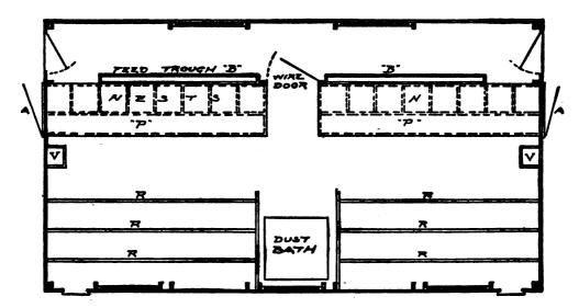
out the cold. A partition three and onehalf feet from the north side of the house forms an alley and the nests are placed against this partition so the eggs may be gathered without going into the henhouse proper. The nest boxes are placed high enough above the floor so the fowls may use the space under them for scratching. The nest boxes are easily removed for cleaning and they are covered with a steep slanting roof to prevent the hens from roosting on them.
