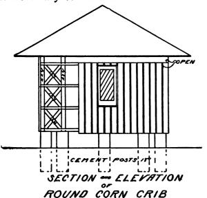
middle. Ordinarily it is not advisable to have a body of corn more than six or seven feet in diameter. By making the inner circle three feet we have six and one-half
