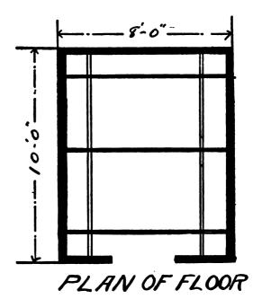
boarding you just take sixteen foot boards and cut them in two in the middle. For the front and back use twelve foot lumber, and the waste pieces work in for roof boards if shingles are used.
