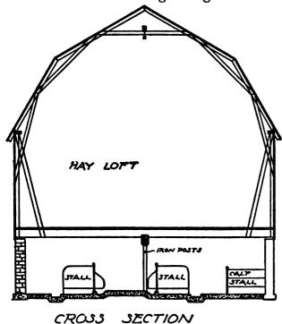
main barn, so that the stock is well protected when out of the barn in severe weather. As will be seen from the drawing, this barn is 40 by 100 feet, and contains stalls for forty-six milch cows, besides loose stalls for calves, dry stock, bull, etc. At the west end is a feed room with
