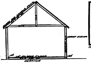
gives an opening ten feet wide, which is very good for small implements, but some binders require about sixteen. The door entering an implement shed must be high enough to let in the highest implements used on the farm, and there must be no cross timbers inside lower than the top of the door. A binder with a reel on takes considerable room.
