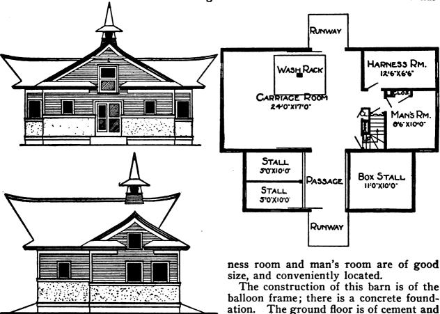
all rooms are cement wainscoted up to the window sills, making the walls water-proof.
