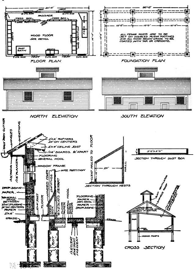
The building is sixteen by thirty feet and contains one general room with a passage, which is also a storeroom for feed, along one side and across one end. All the principal construction details are fully shown in the detail drawings.
