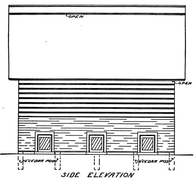
The building is set up from the ground seven feet head room in the middle over about a foot on posts and pens are made the alley and the floor slopes to about five
