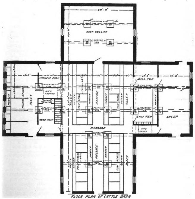
to the ventilation of any stable. The air in a basement stable is seldom as good as it should be. There are two air shafts in this plan with openings near the floor. per floor timbers and joists it is a good plan to make them continuous by building them up with two inch plank so as to tie the building together in both directions.
