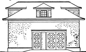
shingle roof. It is set on a foundation of concrete which runs one foot higher than the ground floor, thus avoiding all dampness from the floor and ground coming in contact with the wood construction, which would otherwise soon decay.
