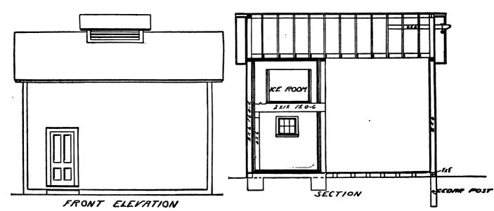
ner wall to make the dead air space as tight as possible. If you have ever undertaken to make an absolutely dead air space you understand the difficulty, or the imthis it is necessary to let the top air out. For this reason a ventilator is built in the roof to encourage a circulation of air between the upper ceiling and the shingles.
