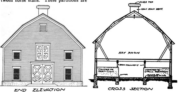
made of reinforced concrete and are rounded down to meet the floor at the bottom which makes a very solid and lasting stall.
