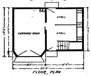
carriage houses, some of which are decidedly homely. A good many of the fancy buildings are too expensive. Here is a comparatively cheap structure, but it is all right for looks and it is a convenient stable to do work in. There is a hay chute which reaches from the loft to the manger below with openings for both stalls, which is a very convenient arrangement and is
