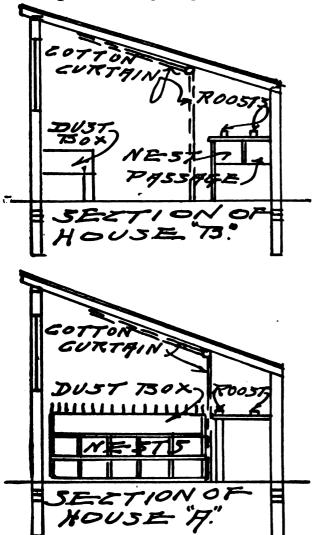
Some poultrymen cover all the openings with cotton and have glass sashes inside that they may slide shut at night or during extremely bad weather. When the cotton ventilators are made right and kept right the air in the poultry house will be good.
