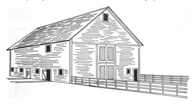
double hinged doors at each end. The large mow above holds ninety to one hundred tons of hay which is taken up inside at the end of the driveway, the floor being afterwards replaced and the section blown full of shredded fodder.
