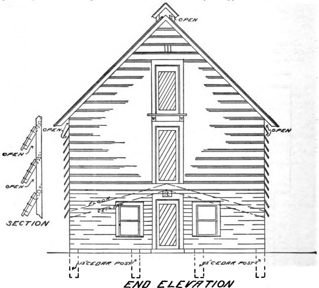
essary to put a slatted partition on both sides of the floor ridge if the house is filled full of corn. There are two windows in each end and the hog doors are hung with pins so they swing either way and the hogs open them going or coming. A pin at the ter which is done by running the alley partitions up to the floor joists above. is very important because the weight of the corn will shove the sides of the building out if the floor is permitted to settle.
