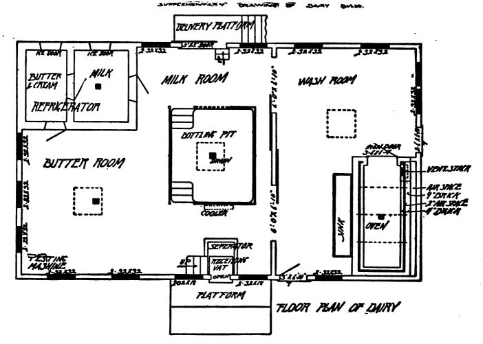
into the separator and after the milk has been separated from the cream it is again mixed together and then flows through the cooler and into the bottling machine, which is located in a pit in the center of the milk room. The filled and sealed bottles are then placed into wooden delivery boxes for immediate delivery or else stored in the refrigerator ready for use.
