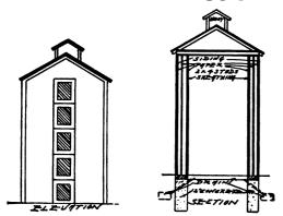
on the outside of these and another set of two by four studding set against them outside of the paper. In this way a wall eight inches thick is made with paper partition in the center.
