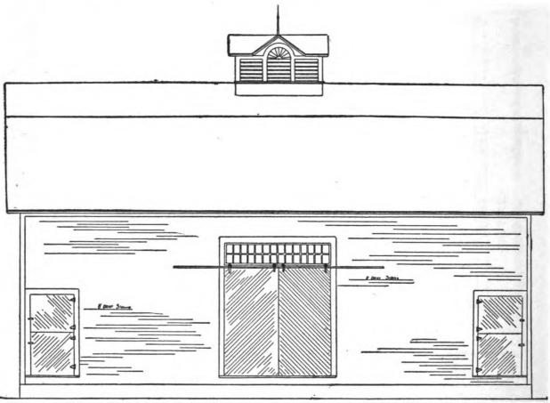
On one side of the driveway is a granary and stabling for three horses with a nine foot ceiling. A third of the barn on the other side of the driveway is made into a cow stable making seven good roomy It seems difficult for some live stock men to understand this phenomenon. The reason is the air circulates more freely when it is warm. The body heat of seven cows in this stable with a low ceiling will warm
