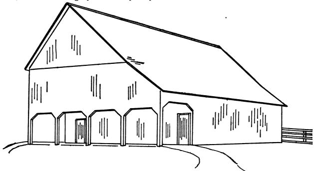
is taken into the mow from outside east end from large door just under comb, and stone pillars with earth floor, and the building is constructed to fit the hill, which
