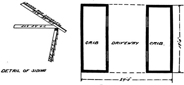
which is placed twenty-four inches apart. It is impossible to get corn enough in a crib of this height to break the slats or shove them out. Corn cribs should not be more than six feet wide because corn will mould in a crib that is too wide.
