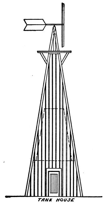
at the top and the shaft must have a bearing, both above the tank and below it so it won't scrape on the pipe. The well and pump of course are directly under the tank in the center of the tower.
