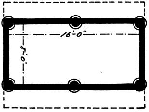
easily covered over, and it is doubtful if they help very much. A better plan is to have the sides carefully constructed and to have the corn in a good condition when it is put in crib. A crib built after this plan may be any length but the posts should not be more than eight feet apart.
