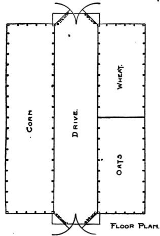
pitch corn or threshed grain. Just ordinary one by four pine strips spaced to ¾ inch are nailed on the outside of two by four studding to make the corn crib, but the wheat and oat bins of course are made tight all around and a little extra work is put on the floor.
