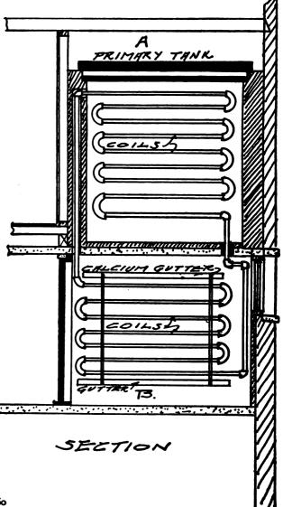
lation whereby the pipe in the lower room is kept cold and the degree of cold is regulated by the size of the cold storage room, the area of pipe surface and the amount of to 40 degrees above zero. Mr. Cooper states that a temperature as low as six degrees has been obtained.
