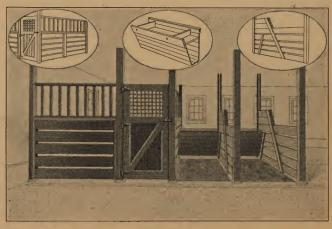
Box Stall, Single or Double Horse Stalls and Mangers. Stall partitions are made of heavy 2-inch planks spaced 2 inches apart. The factory made door for the box stall is furnished ready to hang in place. Prices on material for stalls quoted on request.
