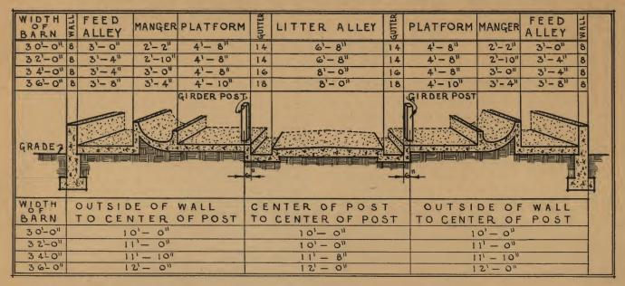
The above illustration shows standard spacing of girder posts and sizes of feed alleys, manger, cow stall platforms, gutters, and cleaning alleys.
