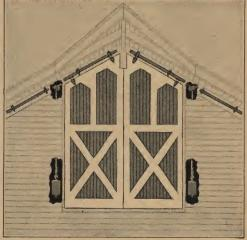
Two kinds of gable hay doors—the gable sliding type illustrated and the hinged drop leaf door—are used on "HONOR BILT" barns. The counterweights for the sliding doors are best made of concrete and are to be furnished by the owner. The hinged door can be easily opened and closed with the aid of the hay carrier. The doors are 9 ft, 4 in. wide by 12 ft, 8 in, high and 1% in, thick.
