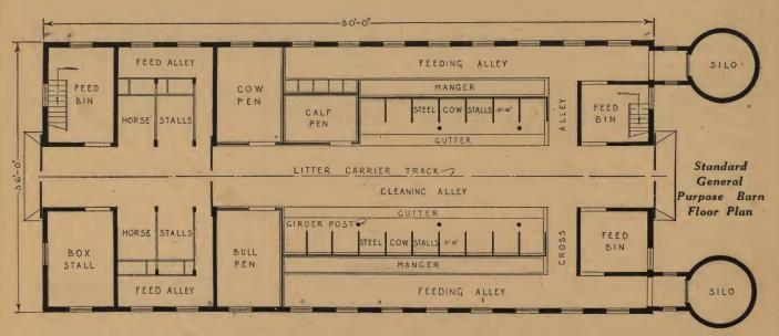
Combination horse and dairy barn floor plan arrangement. This floor plan is suitable for all barns with an 8-foot driveway running lengthwise through the barn.
