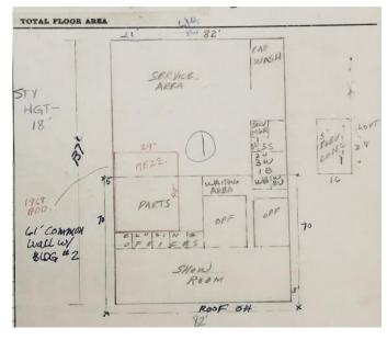
Figure 19. Floor plan of Lake City Dodge, ca. 1968. Note the small size of the show room compared to the service area. Source: King County Property Cards.
