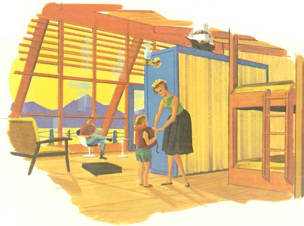
Overlaid plywood serves as combined siding and sheathing on walls. Plywood assures lateral rigidity which this type of structure requires.
