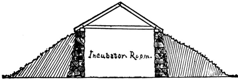
Fig. 203—CROSS-SECTION OF INCUBATOR CELLAR
