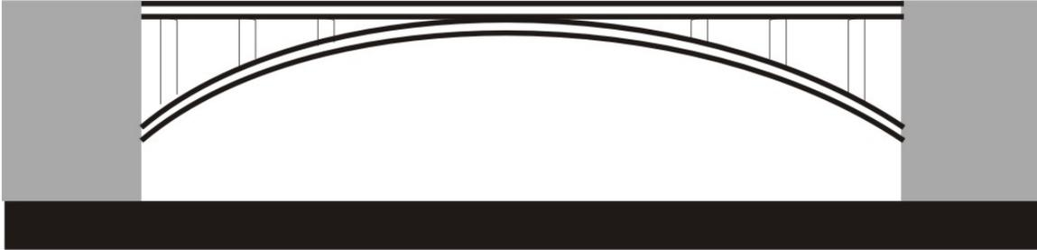
Figure 3-57. Broad River Highway Bridge (1935), State Route 72, spanning Broad River, Carlton vicinity, Madison County, Georgia. This bridge is an example of the open spandrel concrete arch.
