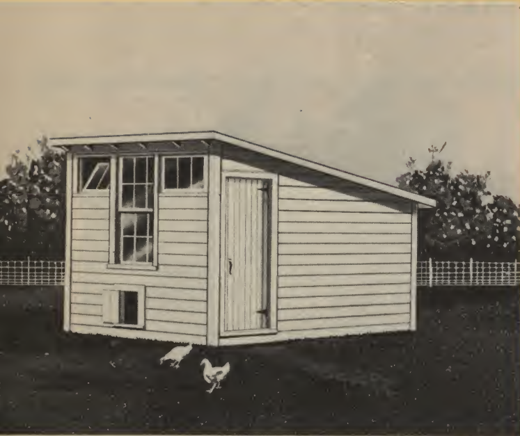
Chicken Brooder — No. 403 ● A type recommended by poultry experts, size 10x12; capacity 350 chicks. Drop siding on exterior walls; roll roofing on roof; lining of 1x4 flooring and ceiling of \frac{1}{2} " insulating board with blanket insulation in the wall and ceiling optional; double floor. Brooder stove should be placed slightly off center toward the rear to permit a wider range of temperatures at floor. Roofing or hardware cloth should be used to keep chicks out of corners.
