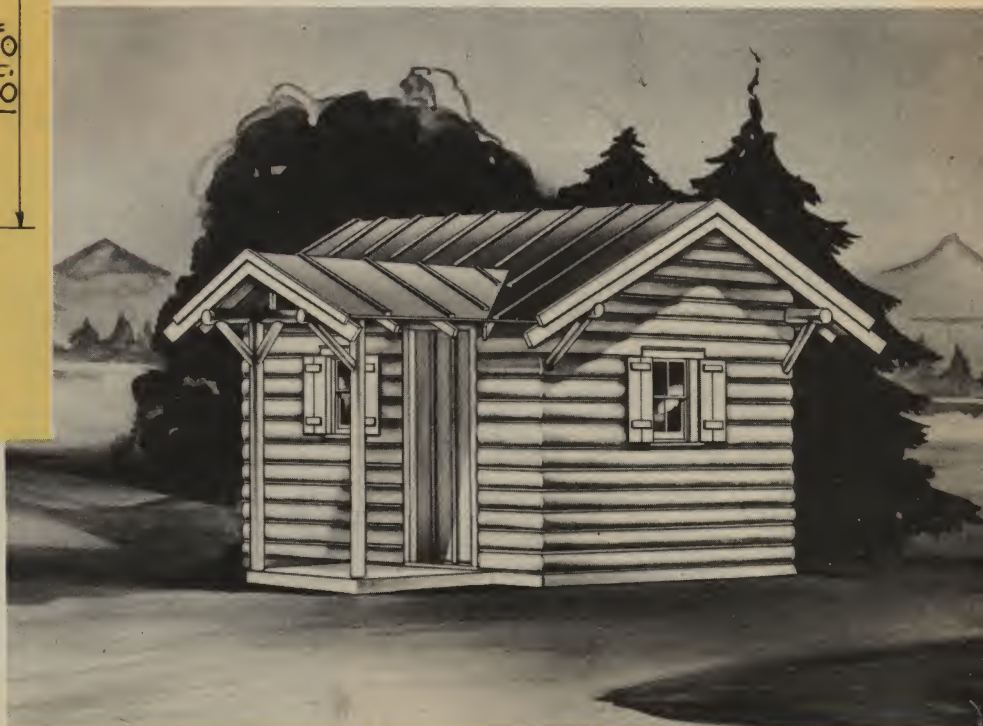
Tourist Cabin—No. 439. A cabin design suitable for a rustic setting, built with walls of log siding. The roof is given a ribbed effect by the use of batten strips over roll roofing. This is a very complete little building for its size and should appeal to the tourist who likes completeness. The floor is of concrete.
