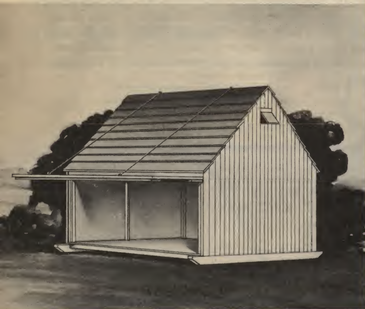
Turkey Brooder — No. 405 ● Ground size 12x12 with 5' studding. 1x4 flooring is used on the walls and 1x12, with a 2" lap, on the roof. Designed for turkeys but may be used for chicks. Capacity 150 poults.
