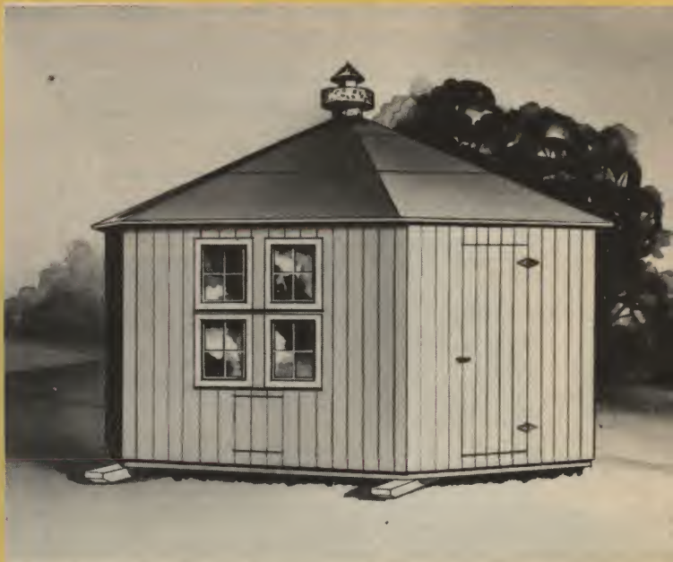
Chicken Brooder — No. 404 ● Hexagonal brooders are preferred by many. This one measures 7' on the side or 14' across the points. The capacity is 350 chicks. 4" or 6" dressed and matched material is used on the exterior with roll roofing on the roof. Floor is double. In cold climates lining and insulation is recommended.
