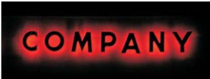
Reverse channel-set letters had neon tubing housed within, or set behind, metal letters. The letter fronts were opaque and backs were open to create a halo of light silhouetting the letter shapes.
