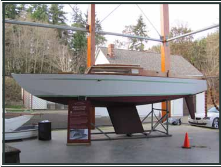
The hull of Thunderbird 1 , a plywood sloop designed by Seattle-native naval architect Ben Seaborn and built by Ed Hoppen, is on display at the Harbor History Museum in Gig Harbor. The 26-foot sloop features a v-shaped hull allowing for the stiffness of multilayered plywood.
