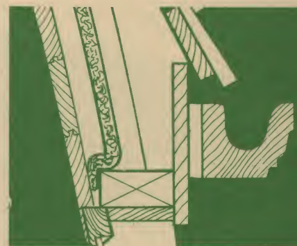
Below — Drainage Gutter.
