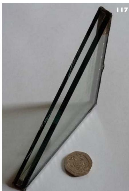
**117:** This slim profile IGU comprises 3mm outer glazing a 3mm gas filled cavity and 4mm Low-E inner glazing giving a total thickness of 10mm.
