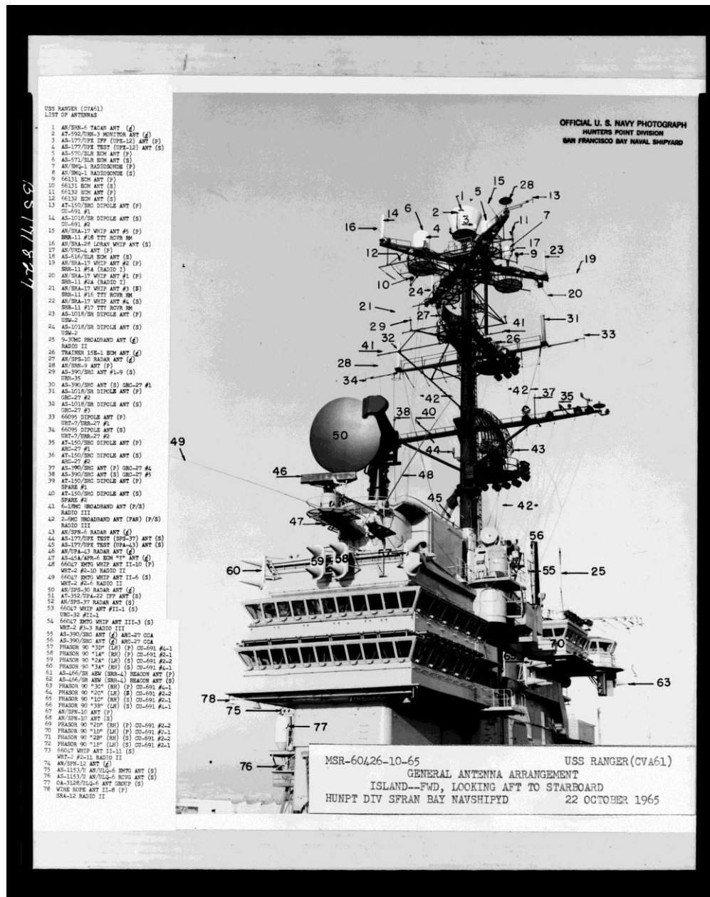
USS Ranger – General Antenna Arrangement: (Photos Courtesy of US Bureau of Ships US Navy, October 22, 1965)
