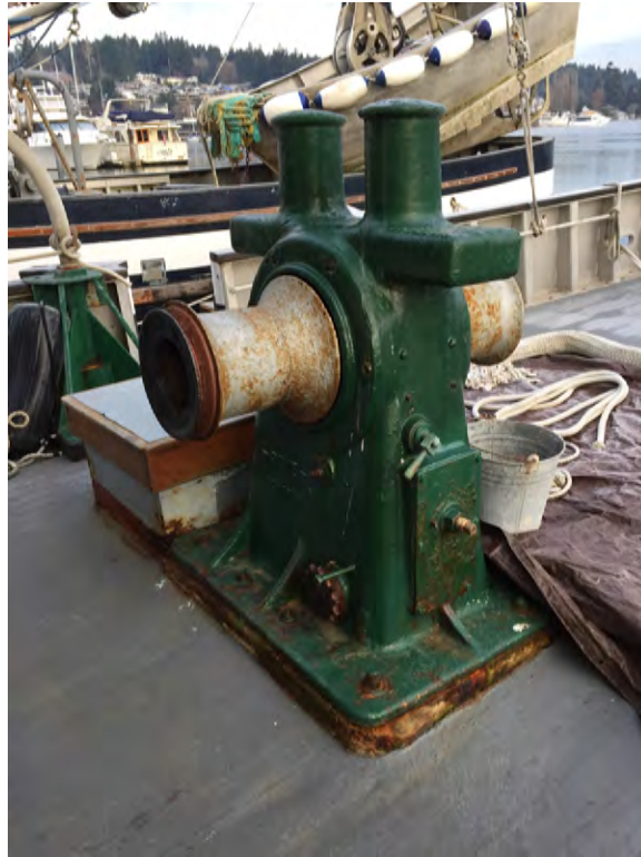
Veteran , former purse seiner. Detail of winch, looking to starboard. One davit visible at left (green). Photo by Susan Johnson, 2015..
